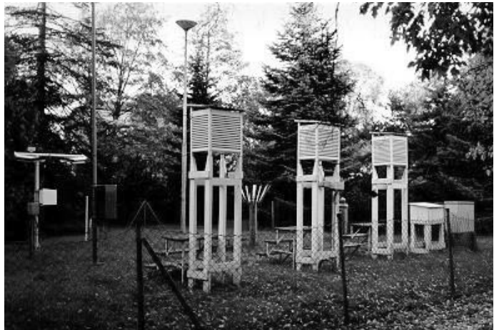
Figure 2 — An example of a parallel observations programme in Helsinki, Finland. Such programmes are required when there are changes in observation systems or site location and comparison data are required to enable homogeneity to be preserved. (Source: Finnish Meteorological Institute, Finland)
